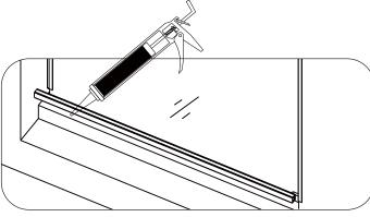
Put the Aluminium Anti-Water Strip (09) in front of the Glass Door (07) on the shower base/threshold, seal it to the shower base/threshold with silicone.
