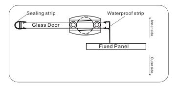
Make sure that the Glass Door with Rollers hangs to the Upper Guide Rail (04), and the glass bottom is inside the Guide Block (11), now adjust glass to vertical and then lock the Safety Pin (15).
