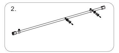
Use the Allen key (19) to loose the screw on the Guide Rail Bracket (02) and Glass Door Stopper (03). Slide the stopper and then the bracket to the Guide Rail (04), use the allen key to tighten the parts to the guide rail temporarily. Disassemble the Glass Bracket (16), insert the bracket core inside the guide rail tube, push it slowly to make the hole on the core match the hole on the tube, then lock the bracket back side with Allen Key(19).
